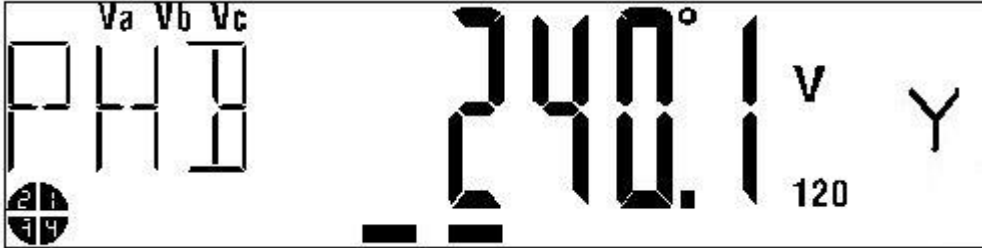
Figure 5.2.2 Sample GyrBox Display on LCD
