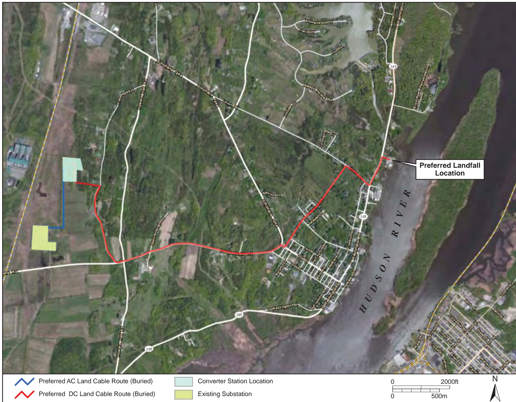
Figure 3. ESRI-derived aerial imagery showing the area of the proposed Northern Converter Station and associated upland Project components.
