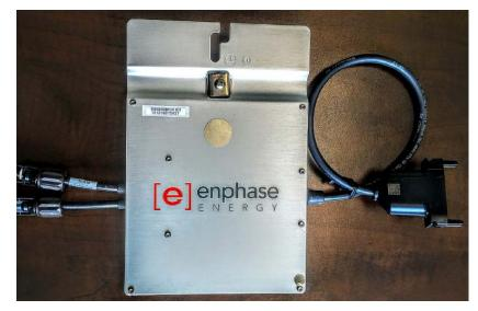
Figure 2-2: Inverter installed on each solar panel
