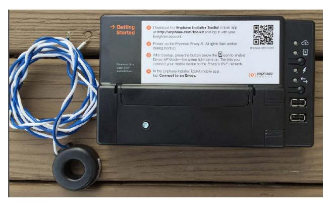
Figure 3-4: An example of an electronic metering system that gets installed inside each residential solar PV system to telecommunicate energy production data to a remote receiver.
