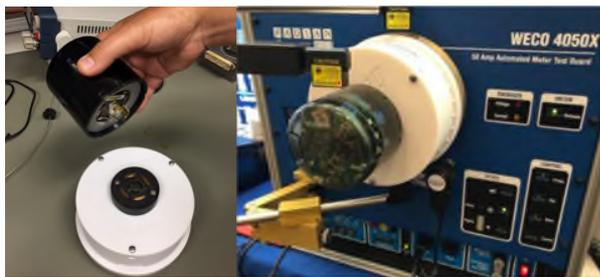
Figure 2. Images of a GE LightGrid® NLC being tested.
