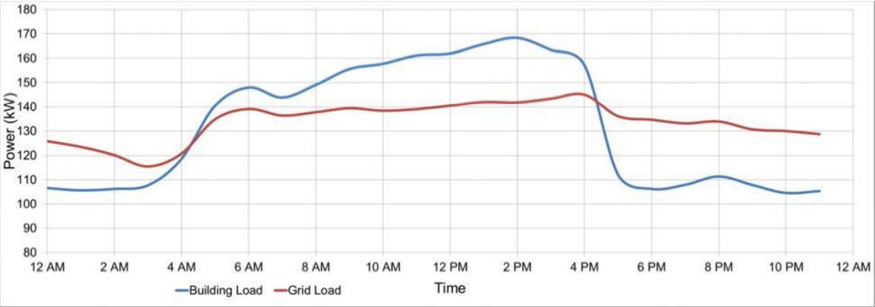
Figure 2. Average hourly circuit peak demand w and w/o presence of battery storage
