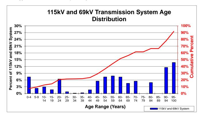
and other capital items are replaced according to a specified timeline. The graph directly below indicates the approximate Transmission System Age Distribution.
